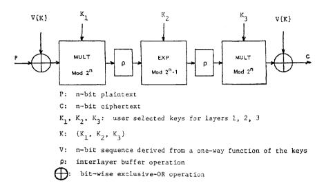
FICURE 4: Block Diagram of the 3-Layered Cryptographic Algorithm.
